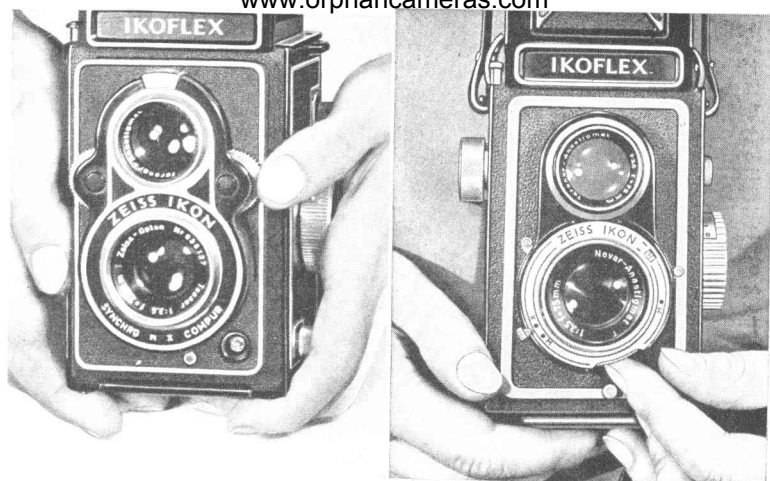
The IkoFlex IIa's shutter speed can be seen from above in the window. Changing the speeds of the IkoFlex Ia.
